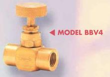
Brass, 1/4" NPT female connections only. Suitable for 600 psi at 300° F maximum; for water, oil or gas service.
