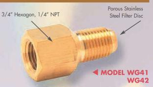
Brass with 1/8" thick micro-metallic stainless steel filter (max pressure 1500 psi) Available 1/4" NPT only. Specify **WG41** for air. Specify **WG42** for water or light oil. **WS41/WS42** Stainless steel body instead of brass.
